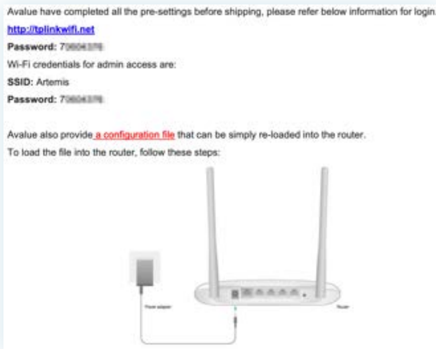
Figure 41 - Default WPA2-PSK password on Avalue RTLS.
